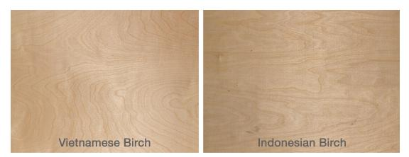
Our import birch is a rotary cut plywood that has excellent maching properties. It's suitable for natural, stained and painted finishes. It has a whole-piece veneer face.
