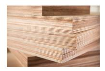
Marine Grade is the highest quality Douglas Fir and Western Larch plywood. It has a variety of uses and is excellent in high moisture applications.
