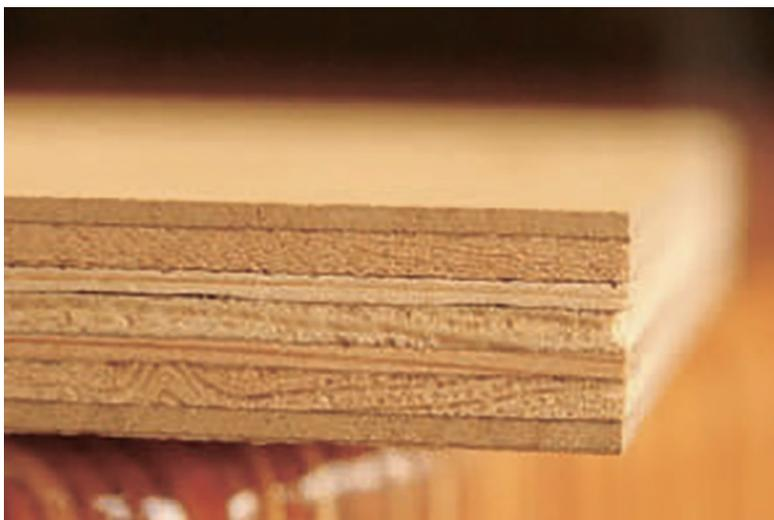
Weyerhaeuser's Ultra-Core™ HDF features High Density Fiberboard surfaces (HDF) fused to a solid core of Structural-1 Industrial Grade Softwood Plywood. The result is a light-weight panel that offers industry-leading structural strength and excellent finishing characteristics.
