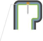
Reminder: All paints will draw away from a sharp edge or corner, regardless of what is being painted: metal, plastic, lumber, plywood, and Armorite. Because the paint is very thin on this area, any expansion and contraction resulting from ambient changes will cause the paint to crack. Rounding edges and corners is highly recommended.
