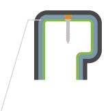
Reminder: All paints will draw away from a sharp edge or corner, regardless of what is being painted: metal, plastic, lumber, plywood, and Armorite. Because the paint is very thin on this area, any expansion and contraction resulting from ambient changes will cause the paint to crack. Rounding edges and corners is highly recommended.
