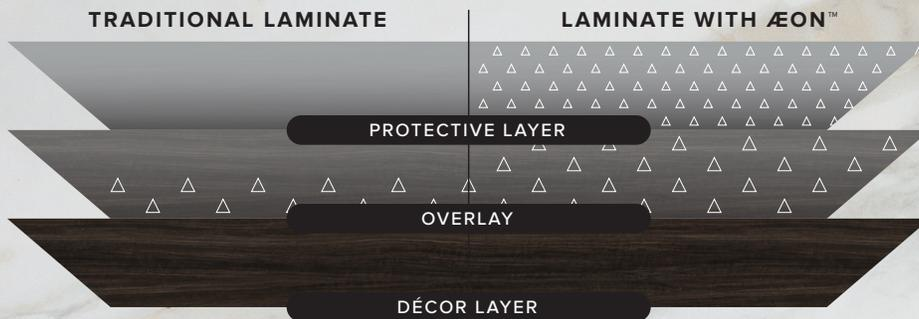
△ = ALUMINUM OXIDE PARTICLES
