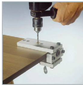
Drill the adjustment hole. Max opening of 1-3/4"
